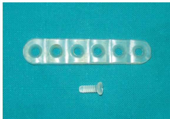
Fig. 1 INION (self-reinforced poly-L/DL-lactide) biodegradable 2.5-mm plate and screw used in this study.
